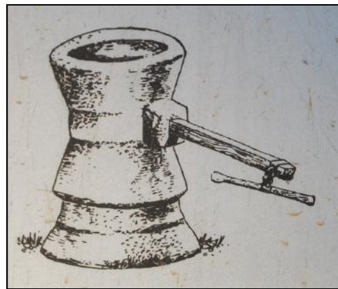
Diagram of the Mill Put Together (A Wooden Bar Fit in the Square Socket and Was Turned by a Donkey)
